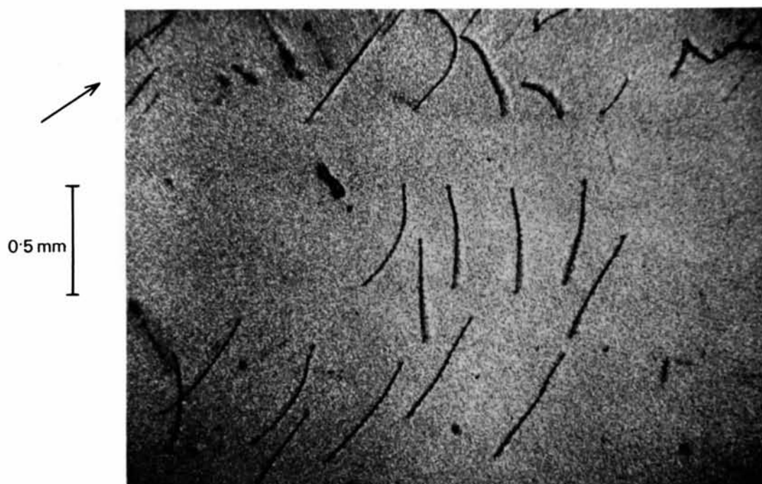
Fig. 4. Traverse topograph of silicon. \bar{1}11 reflexion, Mo K\alpha_1 .
